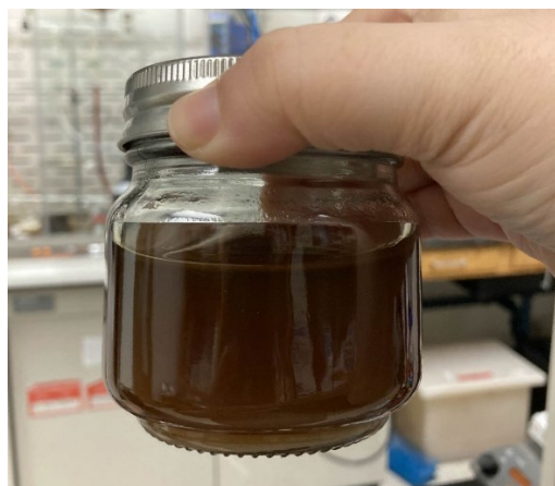
Figure 3: Final alkyd resin. Has honey-like viscosity that can be thinned with oil or solvent into a variety of applications.
