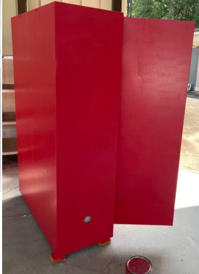
Figure 1: Metal solvent storage cabinet, before and after painting with 50% peanut oil alkyd paint
