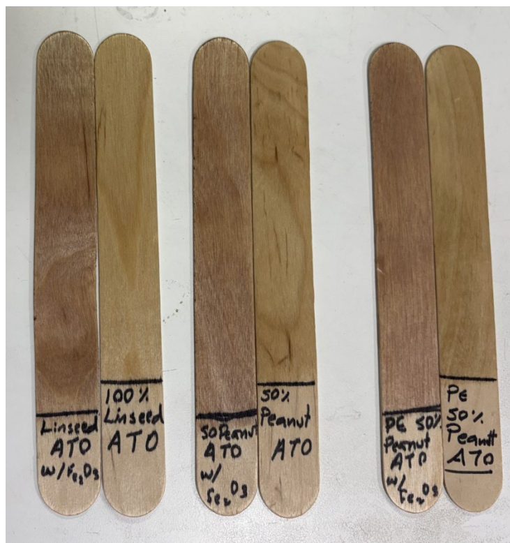
Figure 2: Left: Example product utilizing alkyd in a drying oil formulation. Right: prototype coatings of peanut alkyd drying oil formulations.
