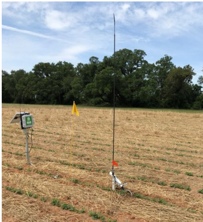
Figure 1. Plot at the SIRP Newton Lateral field in which both Sentek probes with AgSense telemetry loggers (left) and UGA SSA nodes (right) were installed.
