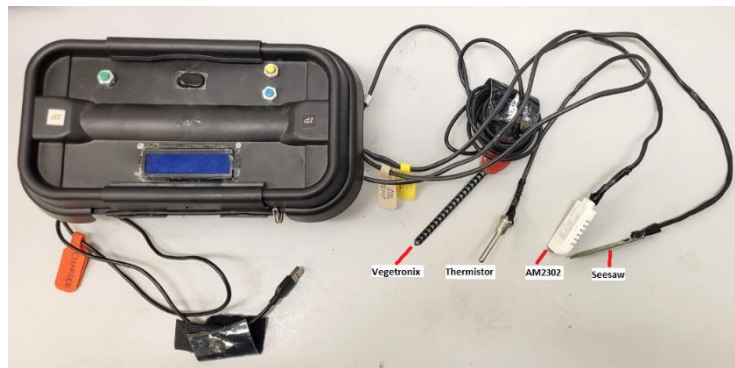
Fig. 1. Soil and Environmental Measurement System V2.A (POEMS) developed at Purdue University
