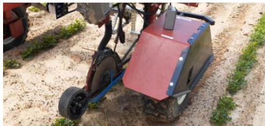
Figure 2 Planter with opening disks, closing mechanism and press wheel
