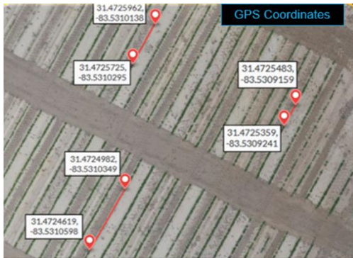
Figure 1 GPS points located at peanut skip locations, table of skip points extracted from aerial image and planter controller hardware.
