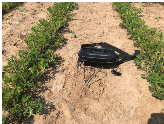
Fig. 2. Portable battery-operated sensing system (First version).
