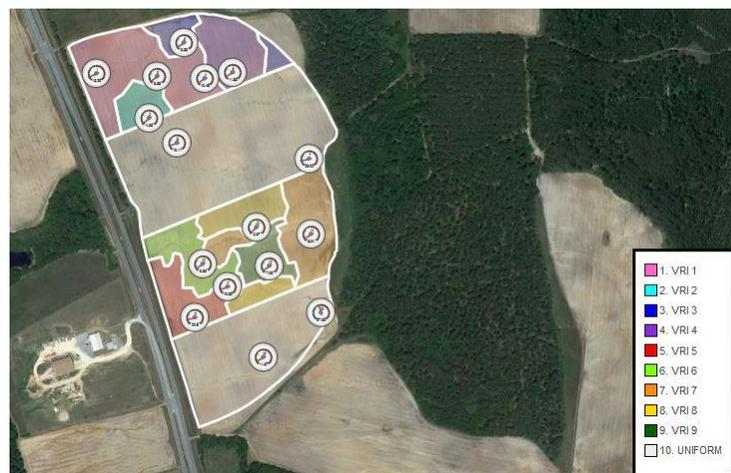
Figure 1. The field used for our dynamic VRI study in 2018. The approach of pairs of parallel conventional and VRI strips will be used again in 2019. The gages indicate the location of UGA SSA sensor nodes.
