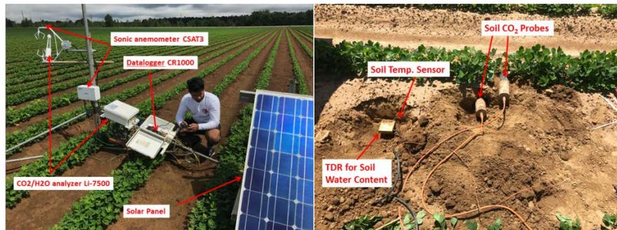
**Figure 1.** (Left) Eddy-covariance system including a fast-response sonic anemometer and an open-path fast-response CO<sub>2</sub> analyzer with solar panel and (Right) soil CO<sub>2</sub> efflux measurements including soil CO<sub>2</sub> probes, time-domain reflectometry and soil thermocouples
