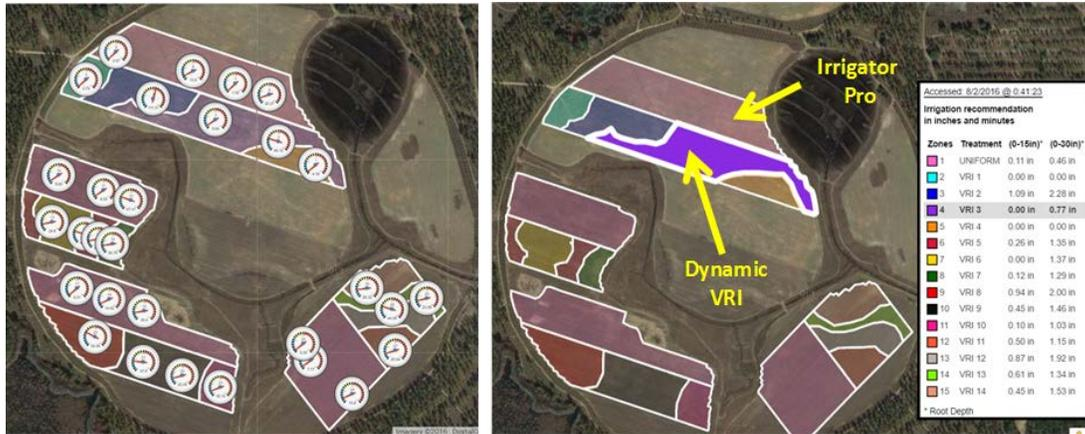
**Figure 1.** Field used for the 2016 dynamic VRI pilot study funded by the Southern Peanut Research Initiative in which we used four pairs of parallel strip. Each pair contained a strip irrigated using dynamic VRI and a strip irrigated using Irrigator Pro. Gages indicate the location of UGA SSA nodes. The legend on the right shows the amounts of water prescribed to each VRI IMZ on 02 August 2016.
